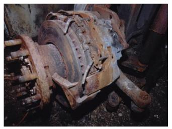
Photo 9: Disc Brake (RH Tag Axle) [Involved]
