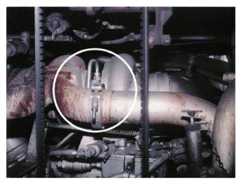
Photo 17: Turbocharger Oil Inlet Line, Series 92
