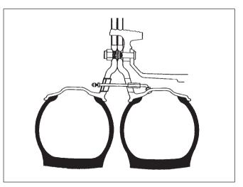
Figure. 6: Cross Section View of Dual Tires
