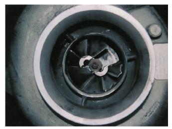
Photo 12: Failed Compressor, Series 60
