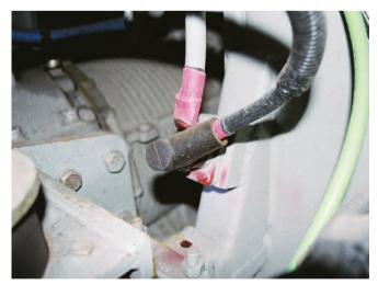
Photo 8B: Bulkhead Connection Bosch T1
