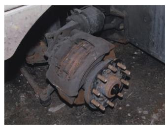
Photo 10: Disc Brake (LH Tag Axle) [Not Involved]
