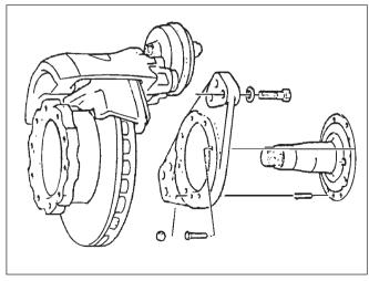
Figure 4: Disc Brake, Caliper, Spider & Spindle
