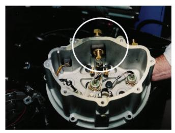
Photo 6A: 50-DN, B+ Stud Insulator
