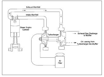
Figure 8: Typical Turbocharger/Intake/Exhaust Schematic
