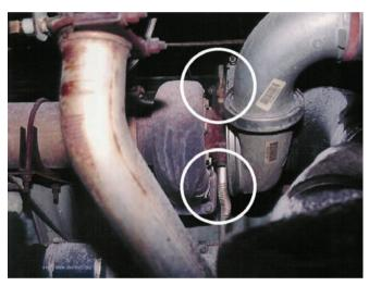
Photo 18: Turbocharger Oil Inlet and Outlet Line, Series 60
