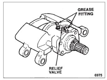
Figure. 5: Rockwell Caliper ADB-1560
