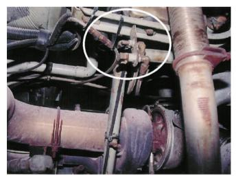
Photo 19: Looped Fuel Lines, Auxiliary Heater
