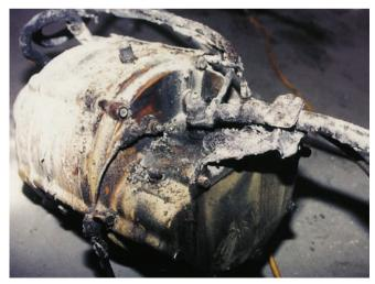
Photo 6B: 50-DN, Result of Failed B+ Stud Insulator
